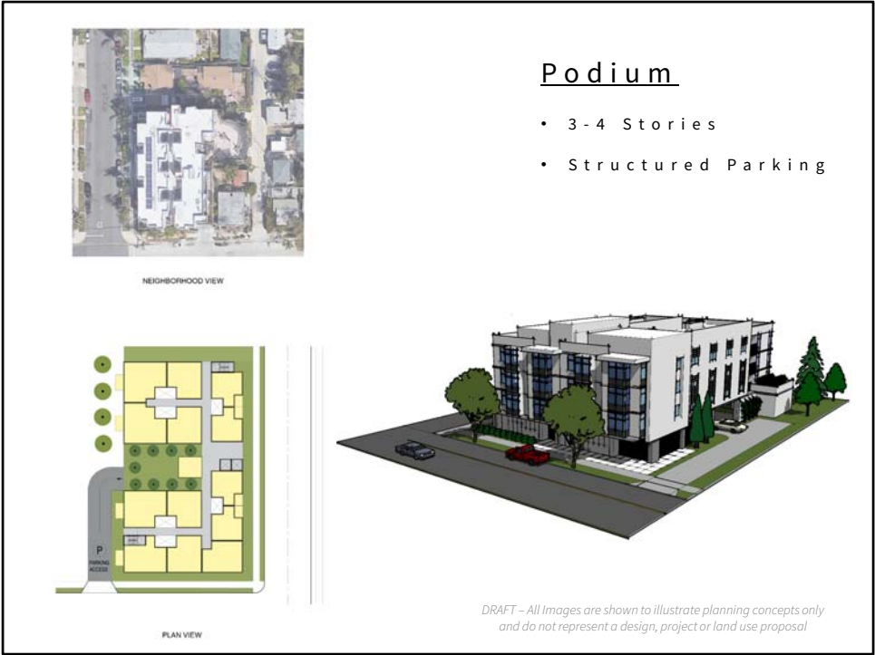
Podium Building Type Typical Plan and 3D view
